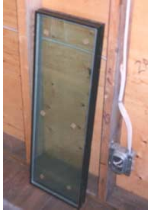
Sealed unit fabricated from salvaged glass - Materials Testing Lab.
