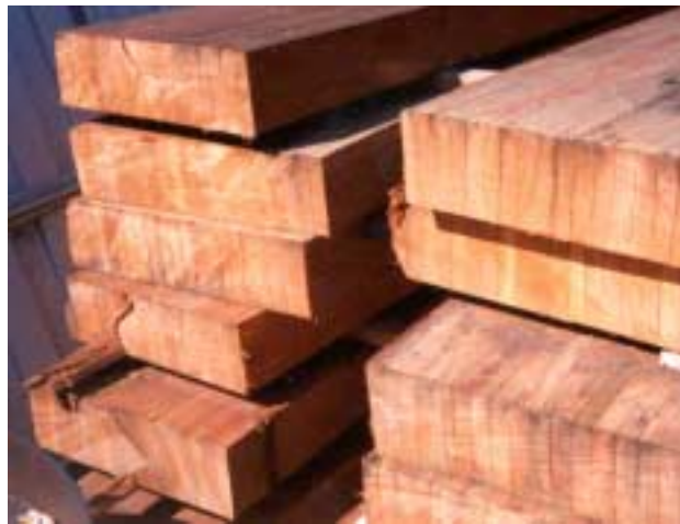
Salvaged Glulam Beams
